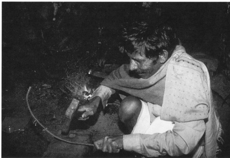
Figure 2: S. Raman making the inner ring for a tablaḱ (frame drum) in the kolēl , or blacksmith's shop. Blacksmithing is one of the traditional Kota occupations, and the smithy is treated as a place of divinity.
